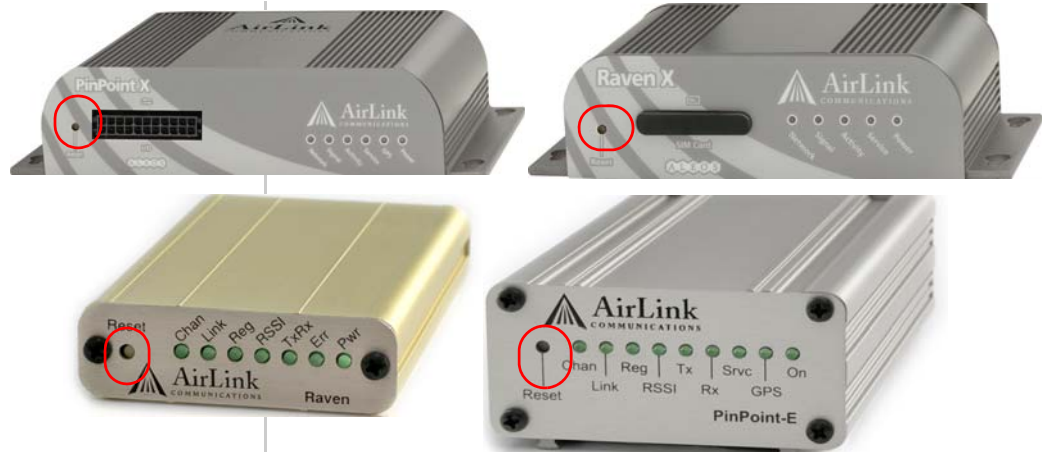
Figure 13-6: Modem Reset button (PinPoint X, Raven X, Raven, and PinPoint-E shown)
